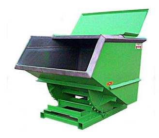
**Description:** 14 gauge center hinged cover with a continuous hinge across the top of the cover. Drain channel under hinge. (Models 680 and larger have 12 gauge Covers) 1/4" neoprene gasket attached to bottom of cover. Cover is watertight. (1) chest handle on each cover. Hopper to have (1)D-ring, chain and snap hook mounted to hopper to hold cover when dumping.
