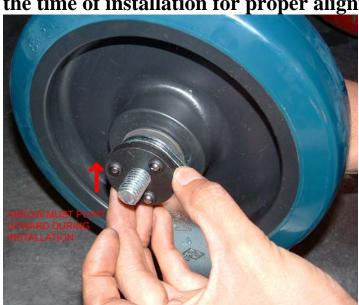
Install brake pedal. 3 channels on the brake pedal will line up with the bearings on the brake plate.
