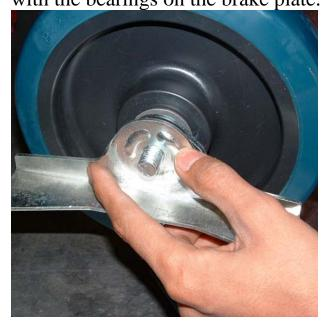
Install spacer washer and then the axle nut.
