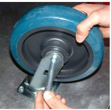
Slide brake plate over the axle with the bearing carriage facing out. The arrow on the carriage must be pointing upward at the time of installation for proper alignment.
