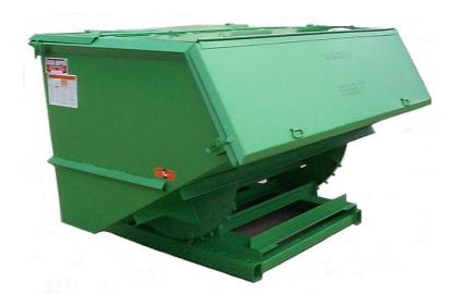
**Description:** 14 gauge Double hinged cover— open nose & back—fixed center cover with a continuous hinge across the top of the cover. Drain channel under hinge. (Models 680 and larger have 12 gauge Covers) 1/4" neoprene gasket attached to bottom of cover. Cover is watertight. (1) chest handle on each cover. Hopper to have (1)D-ring, chain and snap hook mounted to hopper to hold cover when dumping.
