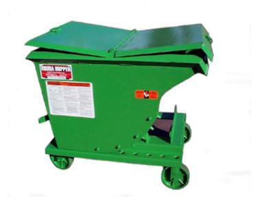
**Description:** 14 gauge center hinged cover with a continuous hinge across the top of the cover. Drain channel under hinge. (Models 680 and larger have 12 gauge Covers) 1/4" neoprene gasket attached to bottom of cover. Cover is watertight. (1) chest handle on each cover. Hopper to have(1)D-ring, chain and snap hook mounted to hopper to hold cover when dumping.
